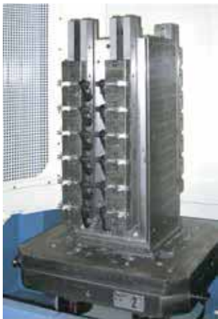
Cubo per piastre riportate con montate piastre e morse MULTIFLEX in verticale Tombstone with modular plates and MULTIFLEX vises vertically assembled
