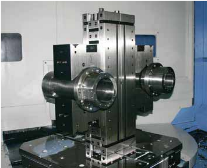
Cubo di morse autocentranti FMS montate in verticale con ganasce prismatiche per pezzi tondi Vise tower made of 2 self-centering FMS vises vertical mounted back-to-back with prismatic jaws for round work-pieces
