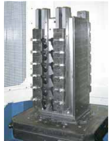
Cubo per piastre riportate con montate piastre e morse MULTIFLEX in verticale Tombstone with modular plates and MULTIFLEX vises vertically assembled
