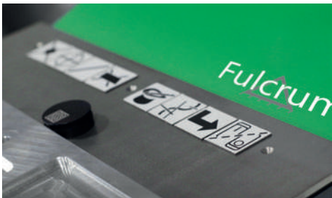
Magnetic buttons allow rapid switching between functions without using the mouse. They can be positioned anywhere on the measuring surface. It is also possible to programme these buttons to perform any function in the Aberlink software.
