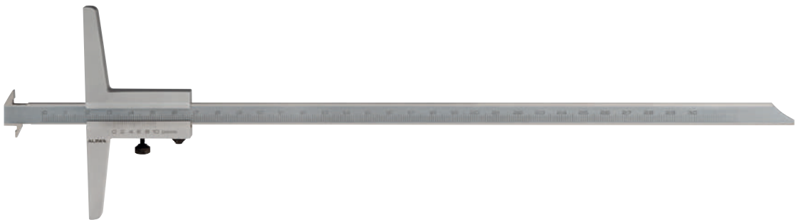
Monobloc caliper with twin feet Nonius 1/20. Readout 0.05 mm. Slide with locking screw.
